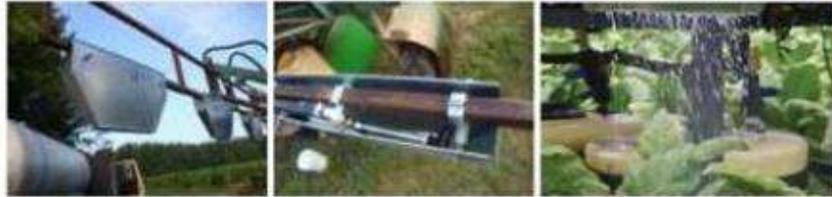
The sprayer hood is used to apply tobacco sucker control products to the crop in a very effective way. The hood will increase the coverage of the sucker control products to the leaf axils for increased control of suckers. This hood simply attaches to your existing sprayer boom and surrounds your existing 3 nozzle cluster.
