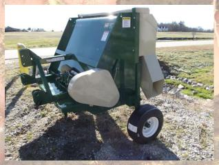
This machine is the ultimate tool for grooming and maintaining plant height. The special designed housing creates a strong vacuum that lifts plants upward before cutting. Blowdown or twisting plant tops, common problems with other mowers, are completely eliminated with this mower. Now you never have to let your plants get too tall. Maintain your plant beds better than ever with the Vac-Master 600.
