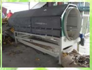
Tobacco Tumbler is used to clean the dried tobacco. It removes the sand from the lugs or first priming's. The Tobacco tumbler also helps to remove any burnt edges from dried tobacco. As the tobacco industry changes cleaner tobacco is going to be a requirement.
