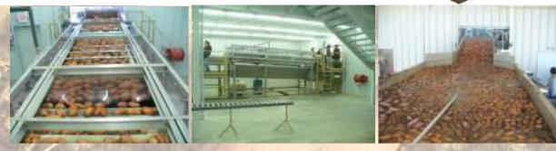
Dump tank with water recirculation system
