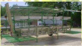
The Sani-Harvest was designed with food safety and efficient packing of produce as some of its top features. All surfaces that the produce contacts are made of stainless steel. This machine can be used efficiently to harvest, weigh, box and load many types of produce such as cabbage, lettuce, leafy greens, and many other types of produce. The Sani-Harvest features a mesh canopy to keep direct sunlight off the workers and the produce.
