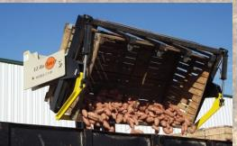
Rotates forward to safely and gently to empty your fragile produce products. Unique bin locking system means no damage to your expensive bins. Rugged and durable design for years of trouble free service. The Bin Rotator is available in sizes to handle 20, 40 and 50 bushel produce bins.
