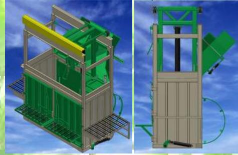
The BaleMaster 5236 provides the most efficient continuous baling process available. It's unique, proven dual chamber design with a single press head provides trouble free baling for years. Its high quality design provides and produces a very neat and square bale. Buy direct from the manufacturer and assure yourself of receiving prompt factory service if needed.
