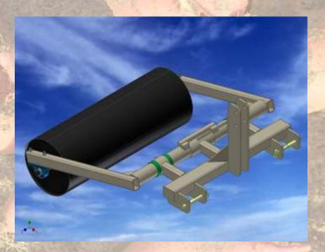
The 3 Point Hitch Bed Roller is a unique piece of equipment that is used to gently apply pressure to seed potatoes. The 3 Point Hitch Bed Roller allows for good potato to ground contact when planting seed potatoes.
